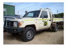
Toyota Landcruiser Workmate 4 x 4 Trayback Utility Model - VDJ79R Date of Manufacture - 11/2008 VIN Number - JTELV71J900009760 Engine - Toyota 4.5L - V8 Turbo Charged Diesel Transmission - 5 Speed Manual Indicated KIms - 212,060 Welded Steel Drop-side Tray Body with Steel Checker Plate Floor BTB - Rollover Protective Frame Towbar, Power Steering, Air Conditioning, Plant Number - VF6071 Please Note: Vehicle has Transmission Issues
