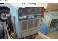
1 Erico Model ESS2500 Electric Arc Stud Welder 3000 Amp, 415 V With Heavy Duty Leads and Mobile Trolley
