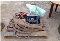
1 Miller Model XMT400CC/CC DC Inverter/Arc Welder With Miller 24V Constant Speed Remote Wire Feeder, Leads and Handpiece
