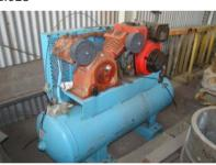
1 **Unbranded Twin Cylinder Received Mounted Air Compressor** Model - VA100 Powered by Unbranded Single Cylinder Diesel Engine Welded Steel Air Receiver 1,800mm x 500mm
