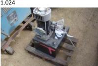
**1 SPX/PT Hydraulics Australia, Hydraulic Power Pack** Model - P5S8A40C60771VDX With Scott DC Model 4BD02249 Electrice Drive Unit 150 Amp/24V/3600RPM
