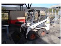
Bobcat - Model 453 Skid Steer Loader Engine: Kubota 3 Cylinder Diesel 4 in 1 Bucket Open-sided ROPS Cab Indicated Hours: 156.4 Serial Number: 515011361
