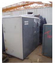
1 Atlas Copco Packaged Rotary Screw Compressor Model - GA37 Date of Manufacture - 2002 7.5 Bar 37 kw 3,000 RPM 1115 KG Serial Number - A11382322
