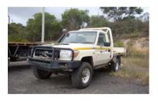
Toyota Landcruiser Workmate 4 x 4 Trayback Utility Model - VDJ79R Date of Manufacture - 03/2007 VIN Number - JTELV71J600001549 Engine - Toyota 4.5L - V8 Turbo Charged Diesel Transmission - 5 Speed Manual Indicated KIms - 225,307 Welded Steel Drop-side Tray Body with Steel Checker Plate Floor BTB - Rollover Protective Frame Towbar, Power Steering, Air Conditioning, Sunraysia Rims Plant Number - VF4459
